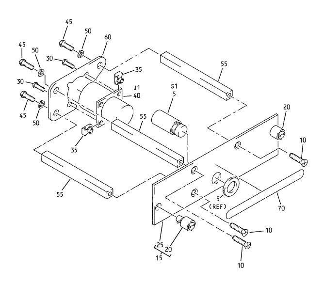
Maintenance Annunciator Light Control Panel Assembly, M2311 Figure 1
